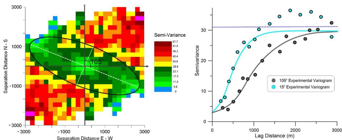
**Figure 4.** Left: The anisotropy map of the gas volume, with the most continuity along the azimuth 105°. Right: Experimental variogram and Gaussian fitted models on the major and minor axis of gas volume anisotropy ellipse
