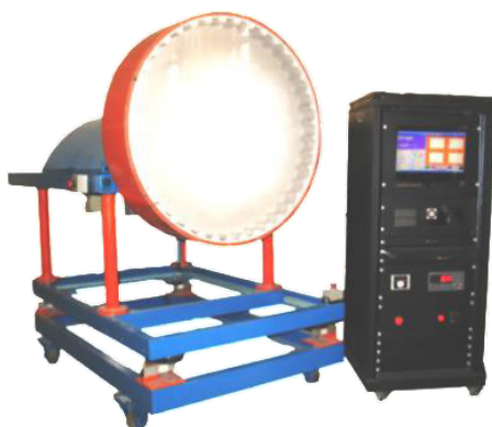
Figure 1. Model mill with control and data acquisition systems
