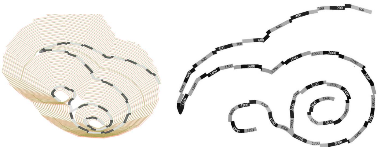
Figure 2. Ramp safety risk zoning in 42 100-meter zones
