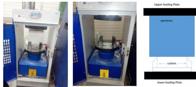
Figure 5. Uniaxial test machine
