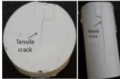
Figure 2. Model under uniaxial compression and Brazilian test
