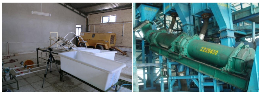
Figure 1. Tri-Flo separators used in this study (left: laboratory, right: industry)
