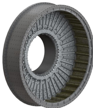
Figure 4. 3D model of the new liners in the Aerofall SAG mill at the Gol-E-Gohar iron ore concentration plant
